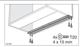
Screw the spacer strip underneath the housing unit sides, flush with the rear wall.
